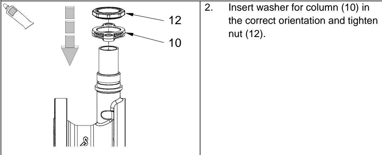
2. Insert washer for column (10) in the correct orientation and tighten nut (12).
