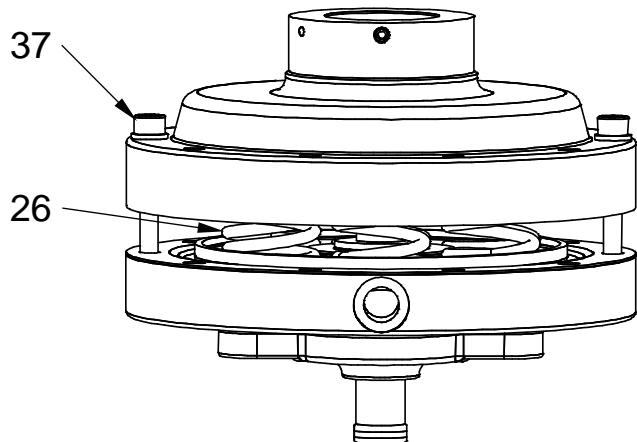
2. Release the actuator springs (26) by evenly unscrewing the last two screws (37).
