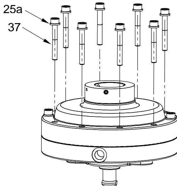
1. Remove screws (37) and washers (25a) until only two opposite screws remain.
