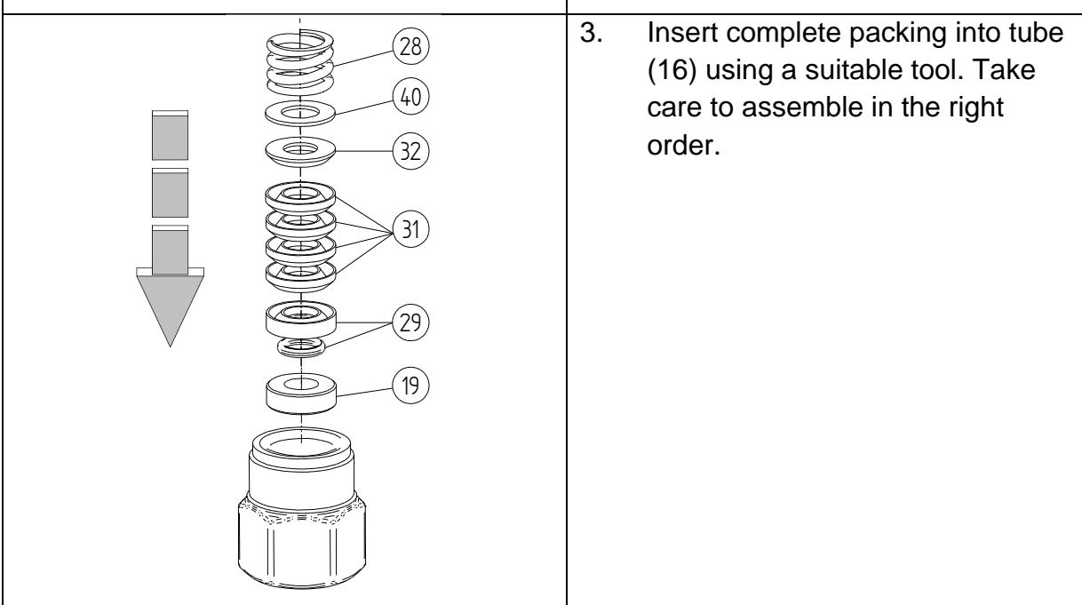
3. Insert complete packing into tube (16) using a suitable tool. Take care to assemble in the right order.
