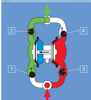
**B** The control valve switches over the air flow into the left-hand air chamber (blue), the right hand air chamber is exhausted. The suction process (see A) now takes place in the right hand pump chamber. Medium (red) is drawn in. Medium (green) is pressed out of the left-hand pump chamber. Valve ball (1) is pressed down and closes, whereas valve ball (2) opens allowing the medium to flow to the outlet.
