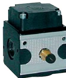
For pumps, which are not primed, the un-throttled opening of the compressed air supply can cause extreme loads on housing materials and diaphragms resulting in a high wear rate. These pressure shocks can be reduced to a minimum by a slow and gradually adjustable pressure increase. The slow start air valve can be used with all DEPA pumps.
