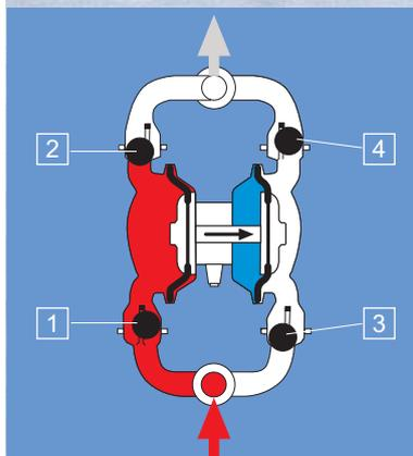
**A** By filling the right hand air chamber with air (blue) the right-hand diaphragm is pushed outwards. This pulls the piston rod on the left-hand diaphragm to the initial position. The valve ball (1) is drawn out of its position, the medium (red) flows into the left-hand pump chamber. At the same time valve ball (2) is seated in a closed position by the vacuum. The left-hand pump chamber fills up with medium (red).
