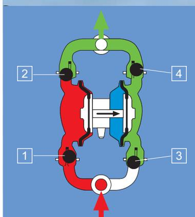
**C** Suction process "A" is repeated with the difference that the right-hand pump chamber is already filled with medium (green). When the control valve switches over the right-hand air chamber (blue) is filled, medium (red) is drawn into the left-hand pump chamber and pressed out of the right-hand pump chamber (green).
