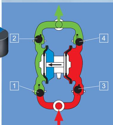
**D** This sequence is repeated in reverse order to illustration C. The left-hand air chamber (blue) is filled, medium (red) is drawn into the right-hand pump chamber by vacuum, at the same time the medium (green) is displaced from the left-hand pump chamber into the discharge pipe.
