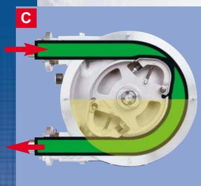
**C** The rotation of the rotor forces the pumped medium inside the hose towards the outlet port on the discharge side. During each opening of the hose a vacuum is created on the suction side ensuring constant suction. It also takes place when the hose is empty giving high suction conditions.
