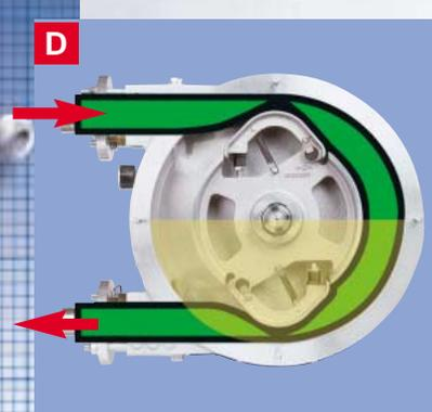
**D** With each rotation the pumping chamber is reformed and the suction capability is renewed.
