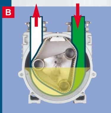
**B** Air from the suction side is pumped over the separator by the turning of the rotor and exhausted outside the pump. This forms a vacuum inside the pump chamber relative to the suction lift, which supports the elasticity of the hose during restoration to its original full cross-section.
