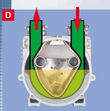
**D** With each rotation the pumping chamber is reformed and the suction capability is renewed.
