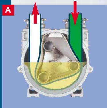
**A** The rotor turns inside the tightly fixed separator. Which is held in the pump housing filled with lubricant. The separator divides the housing into two completely enclosed areas. This means during compression of the pumping hose the suction and discharge sides are hermetically separated.
