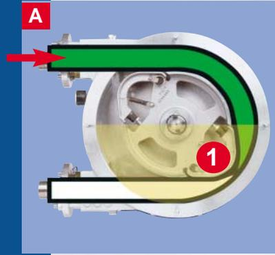
**A** The rotor rotates within the pump housing filled with lubricant and compresses the pumping hose with the sliding shoe (1). This process generates a hermetic separation between suction and discharge side.
