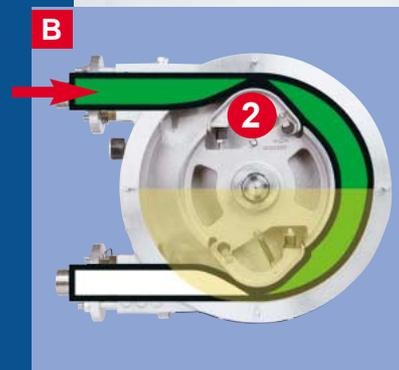
**B** Once the second sliding shoe (2) compresses the hose, a completely enclosed pumping chamber is formed. This volume corresponds exactly to half the pump capacity per rotation. A vacuum is also generated inside the pump housing, supporting the elasticity of the hose allowing restoration to its original full cross-section.
