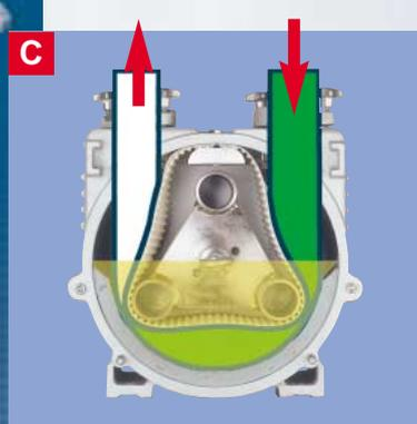
**C** Once the second sliding shoe compresses the hose, a pumping chamber is formed. This volume corresponds exactly to one-third of the pump capacity per rotation. The rotation of the rotor presses the medium inside the hose towards the outlet on the discharge side. During each opening of the hose a vacuum is created on the suction side ensuring constant suction. It also takes place when the hose is empty giving high suction lift conditions.
