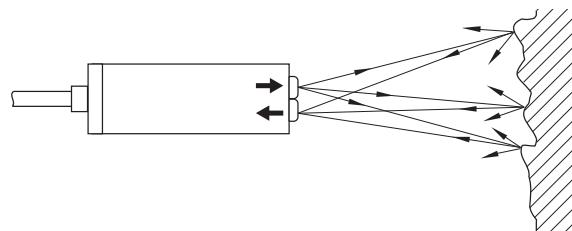
The function of reflex light probes with background suppression is similar to energetic reflex light probes. The difference is that not the quantity but the angle of incidence of the reflected light is evaluated. Thus the dimension, the colour and the surface characteristics of the object hardly influence the switching distance. This is why objects can also be detected without any problem in front of a bright background.
