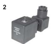
These coils can be mounted with the majority of the Lucifer solenoid valves. This is an encapsulated assembly comprising a coil, integral magnetic iron path and snap-on plug connection. The synthetic material encapsulation provides an effective compact housing, offering full protection against dust, oil, water, etc. Ease of mounting in confined space - offers shock and corrosion protection - simplifies conversion of existing equipment to other requirements, etc.
