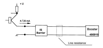
The OFF state is garanteed from a current of 0 mA up to 5 mA. The ON state of the solenoid valve is garanteed when the current is > 18 mA for vibation and shock not exceeding 10 g axially and 20 g radial.
