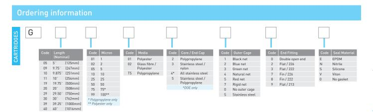
Cartridge lengths are measured over end cap shoulders. For DOE type cartridge lengths are measured over gaskets. Standard elements have diameter 2.7" [68mm]. In nominal lengths of 10, 20, 30, 40 inches. (250, 500, 750, 100mm).
