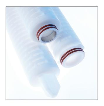
Polyflow II G depth media has been developed for a wide variety of general process applications from fluid clarification to general prefiltration. Its high dirt-loading, random-fibre polypropylene depth media provides consistent particle retention.
