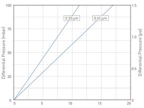
Flow (L / min) for liquid @ 20 °C and 1 cp 10" module Recommended water flow rate of 10l/min/10" module
